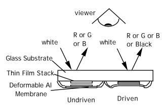
Figure 1 Illustration of the basic structure of a reflective Interferometric Modulator (IMod).
