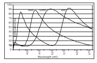
Figure 5 Spectral Reflectance Functions (SRFs) of measured IMod tests at increasing Color/Gap dimensions: green (160 nm), blue (300 nm) and red (400 nm).
