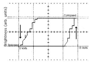
Figure 4 Plot of drive voltage vs. output magnitude revealing hysteresis of the IMod.
