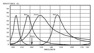
Figure 2 Spectral Reflectance Functions (SRFs) of calculated IMod filter designs at increasing Color/Gap dimensions: black (50 nm), green (160 nm), blue (300 nm), red (400 nm).
