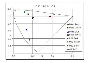
Figure 6 Calculated color gamuts of IMod color display triads compared to P22 phosphorsusing CIE 1976 UCS.
